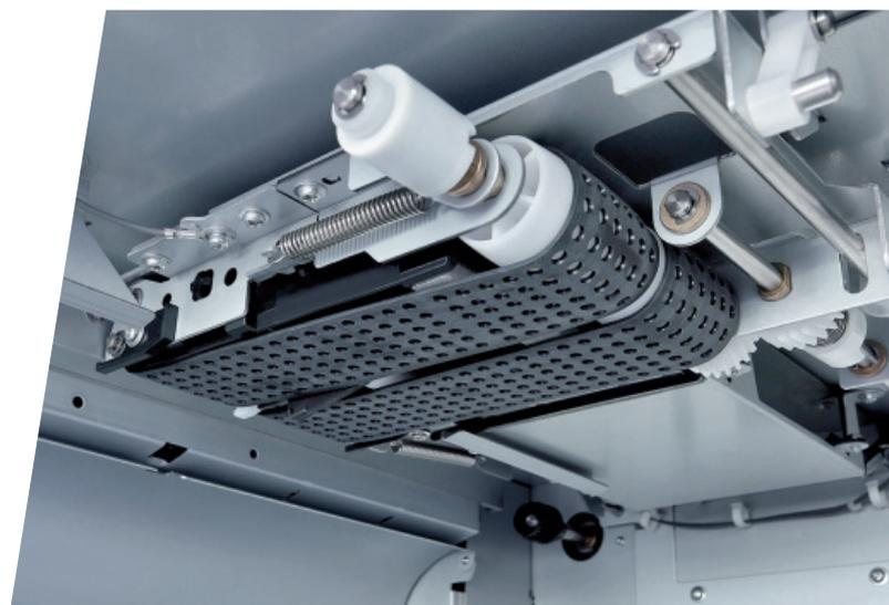
Incorporated vacuum feed technology for both paper feed units
